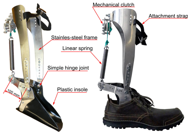
Fig. 1: Our prototype version of the unpowered passive ankle exoskeleton.
